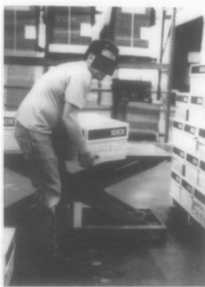
Fig. 2. Repeated sub-failure loads lead to tissue fatigue and failure on the N th repetition of load (or box lift in this example).
